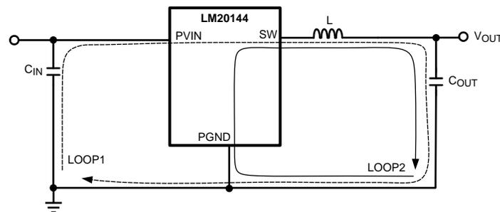
**Figure 36. Schematic of LM20144 Highlighting Layout Sensitive Nodes**
