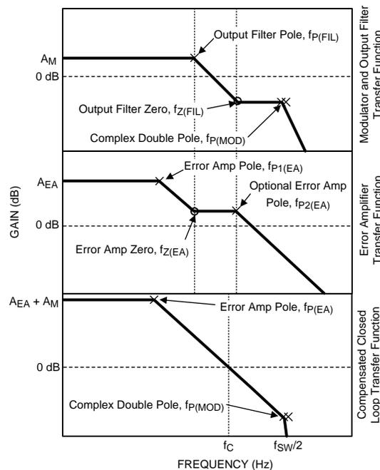
**Figure 30. LM20144 Loop Compensation**
