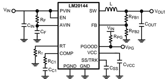
**Figure 28. Typical Application Circuit**
