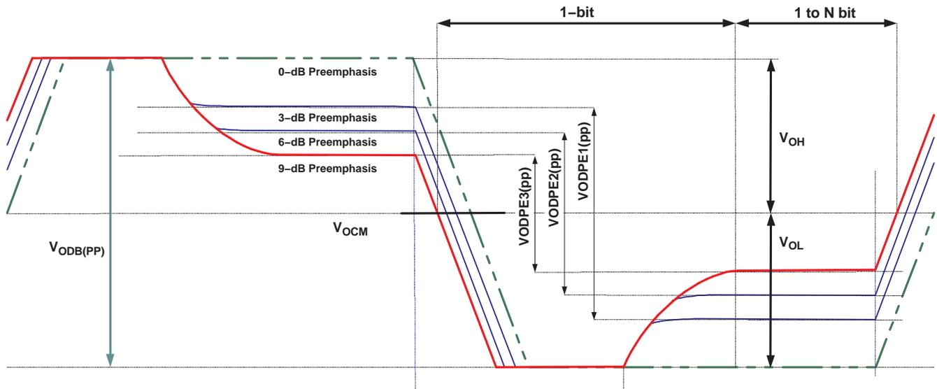
Figure 3. Preemphasis and Output Voltage Waveforms and Definitions
