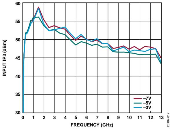
Figure 17. Input IP3 vs. Frequency over  $V_{CTRL}$
