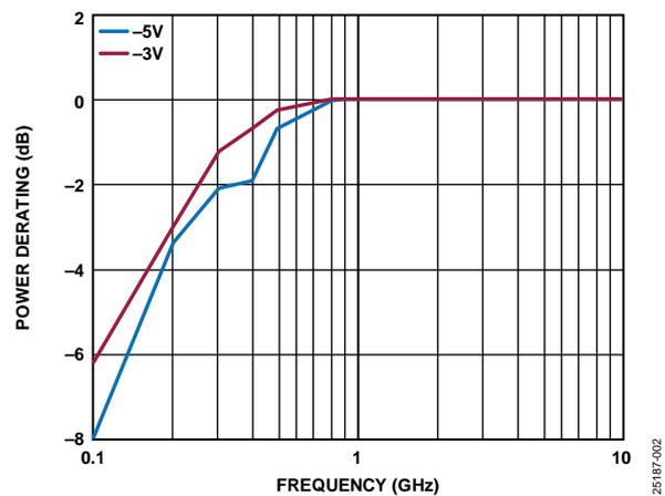
Figure 2. Power Derating vs. Frequency over V<sub>CTRL</sub>, Low Frequency Detail, T<sub>C</sub> = 85°C
