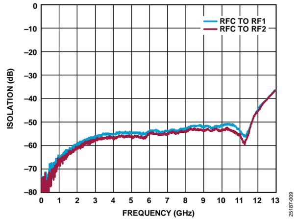
Figure 10. Isolation Between RFC and RFx vs. Frequency
