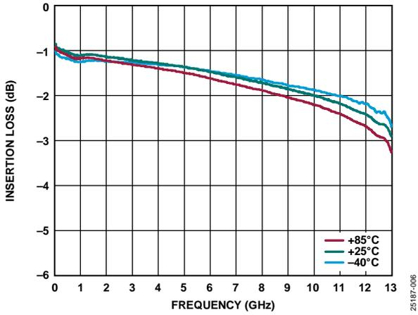
Figure 7. Insertion Loss vs. Frequency over Temperature
