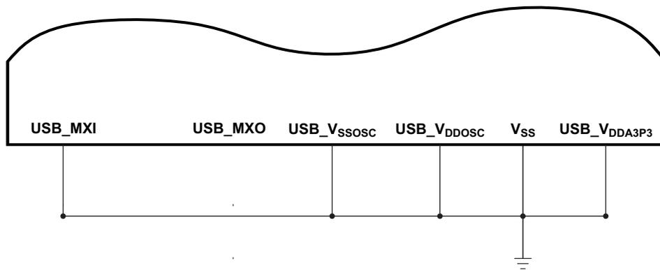
Figure 5-15. Connections when USB Oscillator is Permanently Disabled
